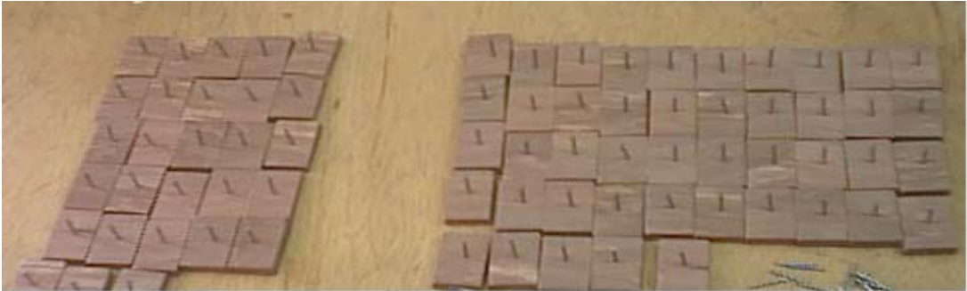
Here you see the Janko key-tops ready prepared (sanded & nailed) for painting!
